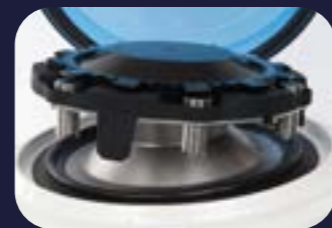
Metal tubes Up to 6 tubes (6mL accessories) Used for very hard samples
